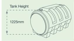
There should be a flat area around the tank inlet aperture. Remember, if fitting i-Track to a bunded tank (double skinned), measure from the inner surface. This illustration is for example only. Always measure the tank as sizes vary.
